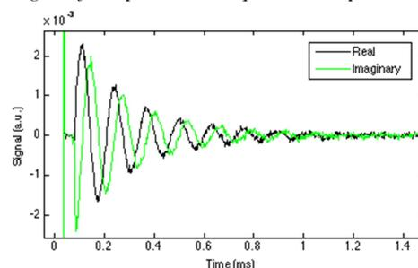
**Figure 2:** A pulse-and-acquire FID recorded by the USRP1.
