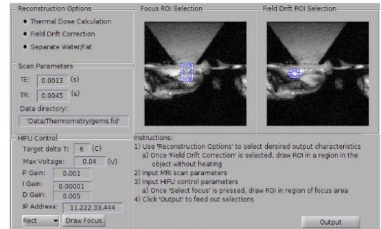
**Figure 2:** Graphical user interface for the control and monitoring software.
